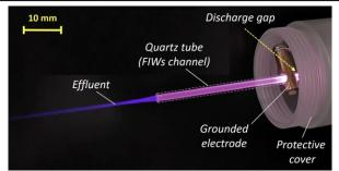
**Fig. 1**. A photograph of the ns-jet discharge working in a pure He gas flow. The high voltage electrode is located inside the protective cover on the right side. [5]
